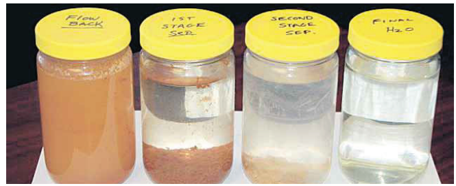
Four jars documenting the stages of flowback treatment, from chemical breaking (far left) to clear water (far right).
