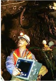
GPR scanning of an underground mine roof for hidden delaminations
